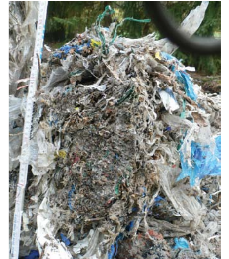
The rags can have a length of up to 15 m and a diameter of up to 800 mm. ▶
