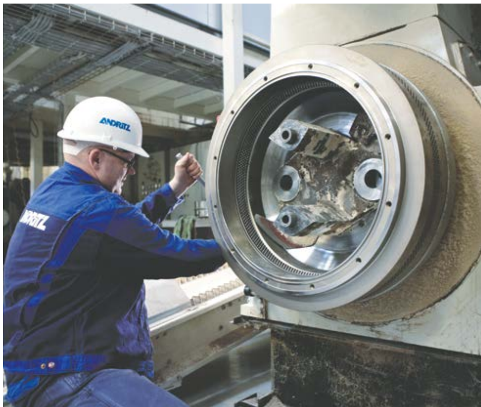
▲ Pellet mill maintenance
