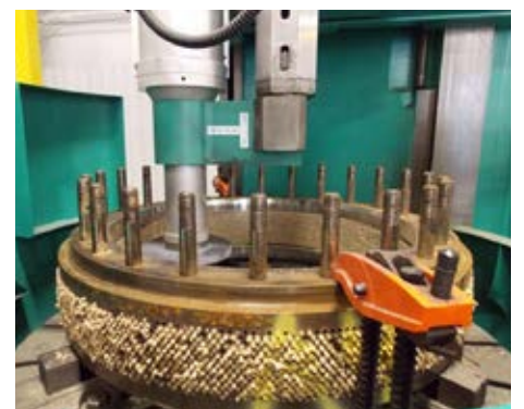
▼ Die refurbishment in Savannah, GA, USA
