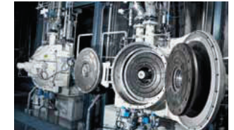
▲ TwinFlo refiners for optimum fiber development in the stock preparation process.
