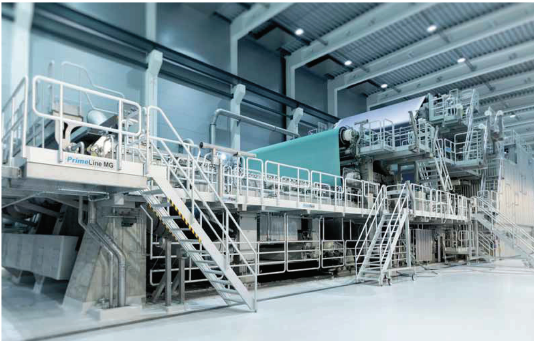
▲ The PrimeLine MG paper machine has a working width of 5.4 m and features a number of technical highlights.
