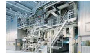
▲ The gigantic heart of the machine – the PrimeDry Steel Yankee – is the largest in the world.
