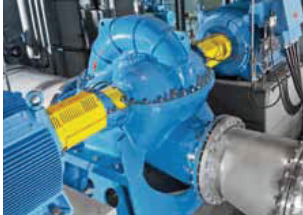
▲ The ANDRITZ headbox pump for PM2 operates at an impressive 92% efficiency.
