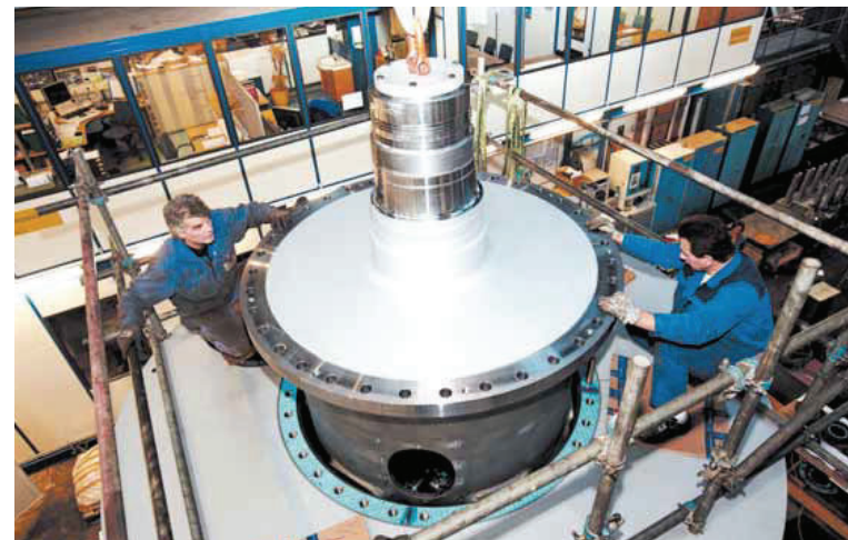
Assembly in the ANDRITZ workshop in Graz: lifting the hollow shaft into the dryer shell. ▼
