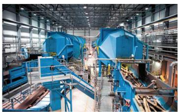
The brownstock washing system includes new pressure diffuser (left) and new two-stage
