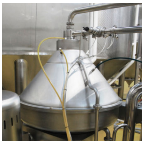
▲ KO 2 , gas purging to sealing chamber
