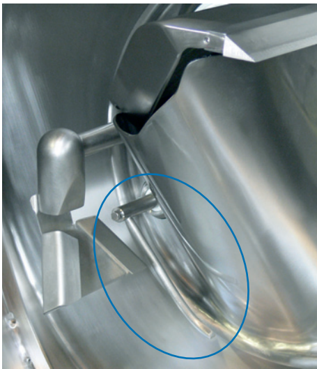
▲ Installation of FCA (Feed Control Analog) in centrifuge
