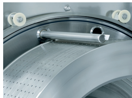
▲ Pneumatic removal of residual heel
