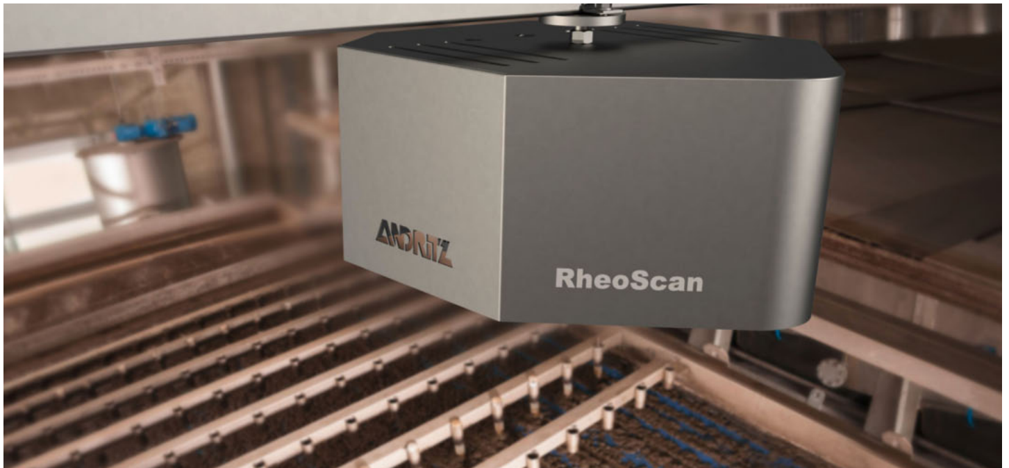
▲ RheoScan installed at a gravity belt table
