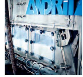
▲ To produce KROMOPAK, the conventional vacuum formers on PM3 had to be replaced by a fourdrinier wet section. Adding the new PrimeForm HB hybrid former on the filler layer enabled the correct level of dewatering and improved formation.
