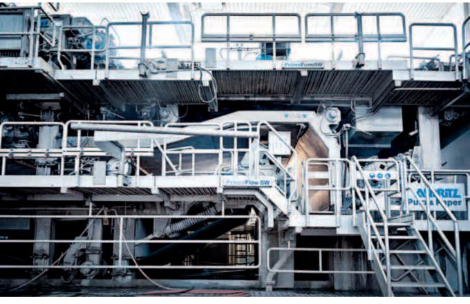
ANDRITZ succeeded in executing the wet end rebuild in only 26 days. The existing cylinder mold formers on PM3 were replaced with a three-layer fourdrinier (PrimeForm SW) which included three new PrimeFlow SW headboxes. The PrimeForm HB is utilized for filler layer dewatering. The existing press section was upgraded with a pick-up roll to allow a closed web run to the press section.
