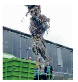
Waste paper is usually delivered to paper mills in pressed bales held in shape by wires. The stock preparation process generates rags that comprise wires and other rejects. Rejects are all those materials that are not paper, such as plastics, textiles, and metals.
