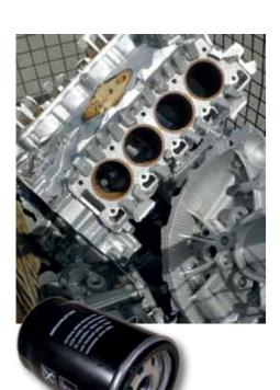
Replaced oil filters from cars and trucks are classified as special waste worldwide. However, they consist of some 60% metals (mainly iron). The oil makes up around 20% of the material mixture. The actual paper filter, rubber sleeves, and other plastic parts make up the remainder.
