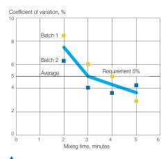
Homogeneity of tracer in 10g samples of hog feed mixed in an ANDRITZ HPB 6000 batch mixer
