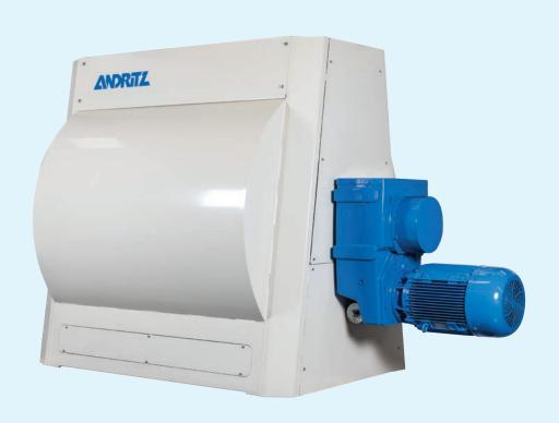
The ANDRITZ OptiMix paddle mixer is fast and efficient. The OptiMix is self-cleaning because the rotor changes direction between each batch and all surfaces are kept clean as a result. The nozzles are placed directly in the inlet, en-
