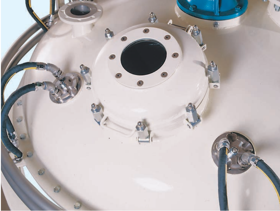
▲ Inspection door hinged for quick opening provides easy access to coater. Sight glass allows visual inspection during operation.
