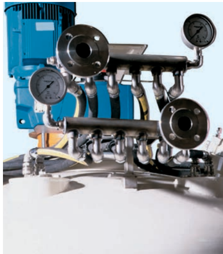
◀ Liquid manifolds ensure even distribution of the liquid to the nozzles independently of the flow rate.
