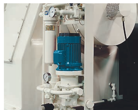
▲ Pellet mill oil cooling
