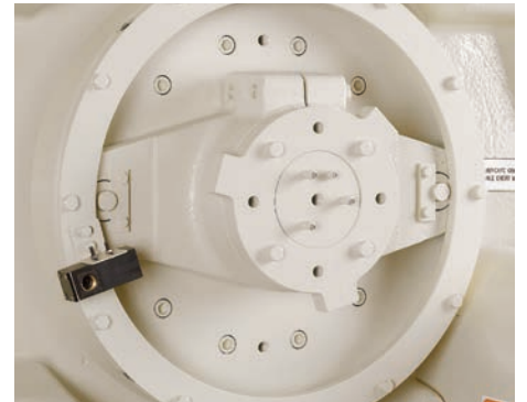
▲ Shear pin overload protection
