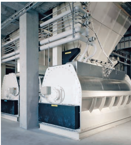
◀ CM series for pre-conditioning with addition of liquids and steam, providing optimum mixing and retention time.
