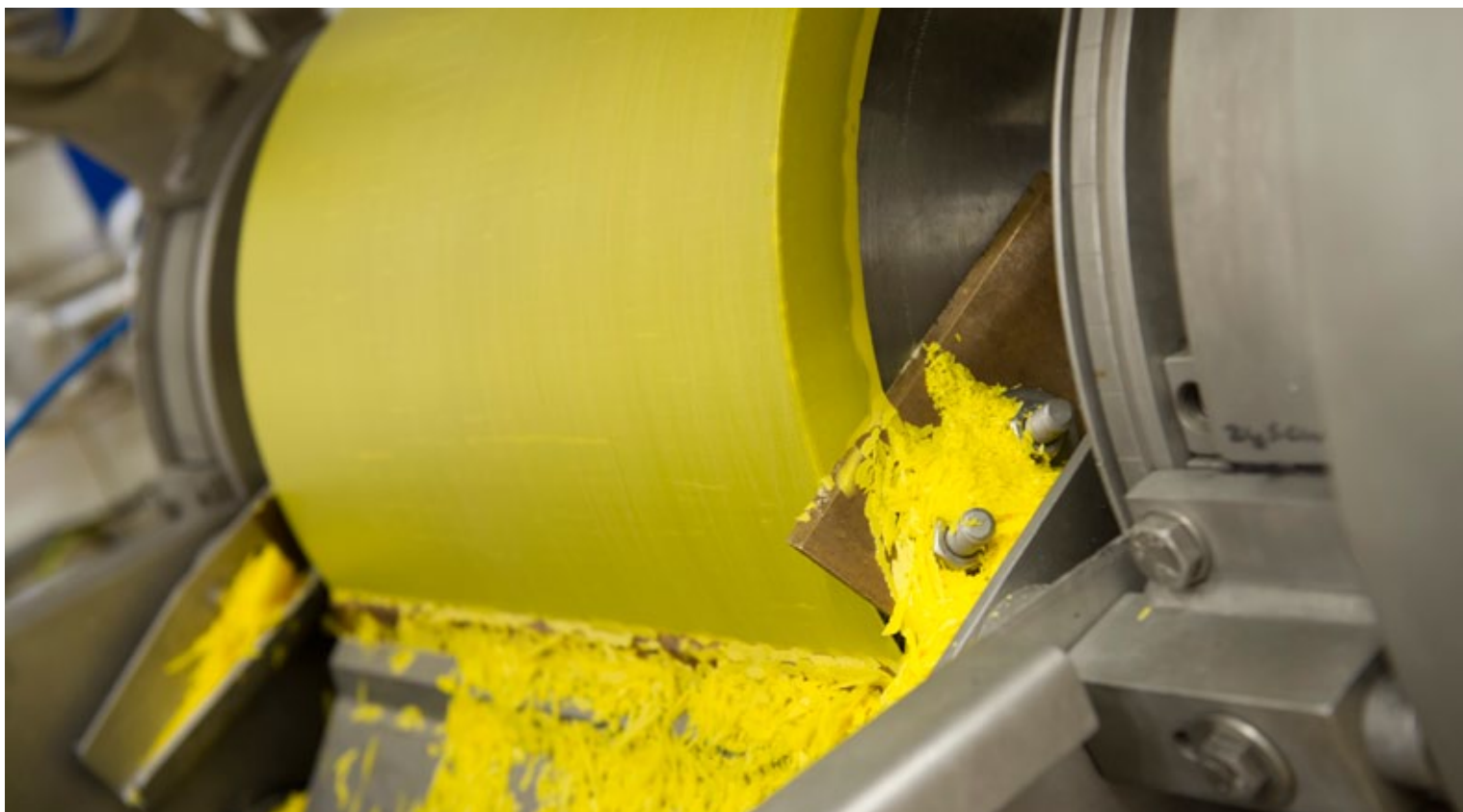
▲ Flake test in our pilot plant
