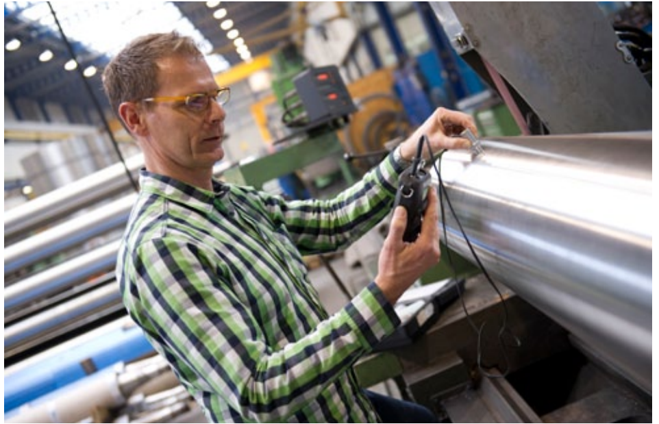
▲ Wall thickness measurement
