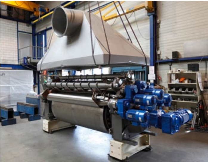
▲ Drum dryer with vapor hood
