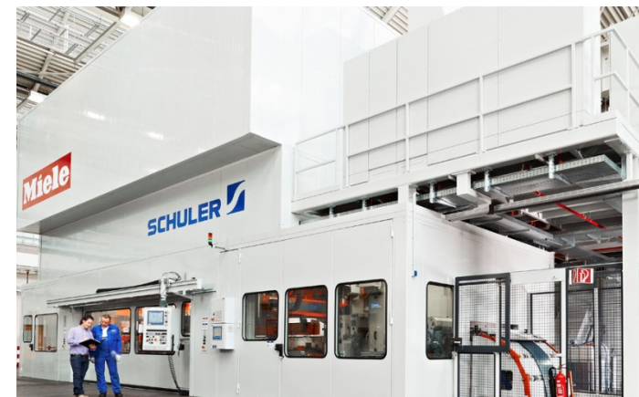
▲ Schuler successfully started up a 1,600 ton servo press for Miele, Germany. Miele increased the output by up to 50% with the new press.
