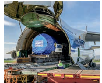
Turbogenerator, USA Transport of a 90-ton turbo generator with one of the world's largest airplanes – an Antonov 124 2013
