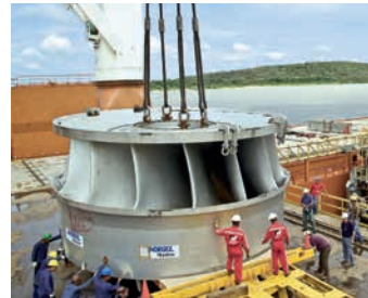
Simón Bolívar (Guri II), Venezuela World's largest Francis turbines (5 × 770 MW) for the largest hydro-power plant in Venezuela 2006
