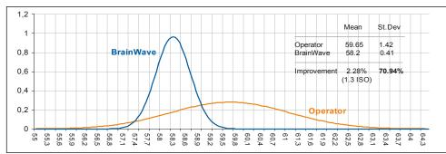
▲ Figure 1: Normal distribution, operator versus BrainWave (final LAB brightness)
