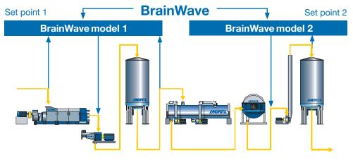
▲ How BrainWave models fit into a process system
